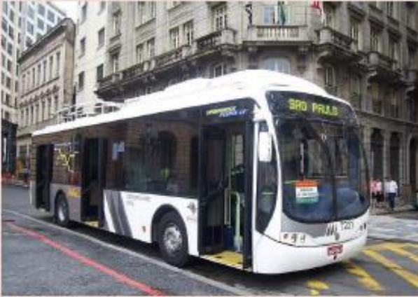
EMTU low-floor trolleybus in São Paulo provides three door boarding.
