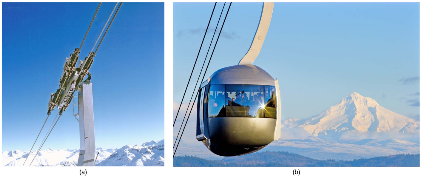
Fig. 1. An aerial tramway:(a) cable configuration; (b) a cabin; (The Doppelmayr Group 2011)
