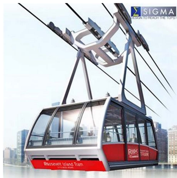
Fig. 3. Cable and cabin configuration of a dual-haul aerial tramway; sourced with permission from the Roosevelt Island Operating Corporation (RIOC 2011)
