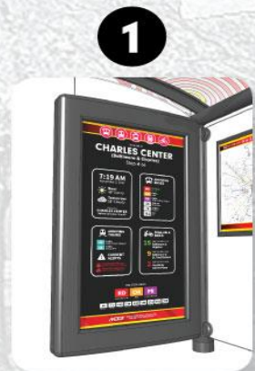
1 Ad Panel with LCD Screen on Inside Outside contains conventional backlit wayfinding panel
